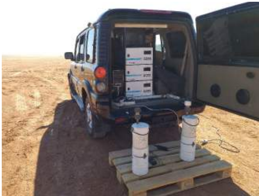
Figure 5-14 Photo of AQ monitoring equipment (left) and ozone colorimetric gas detection tube (right).
