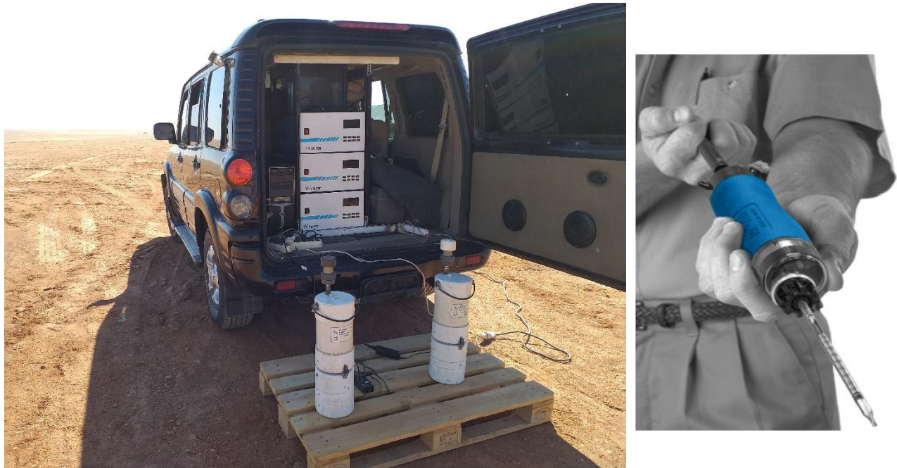
Figure 1: Photo of AQ monitoring equipment (left) and ozone colorimetric gas detection tube (right).
