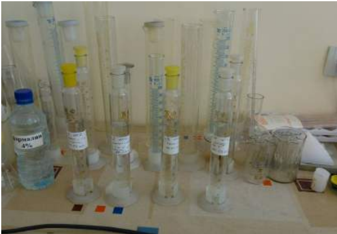
Settling samples of phytoplankton and bringing the volume to 100 ml (5 days)
