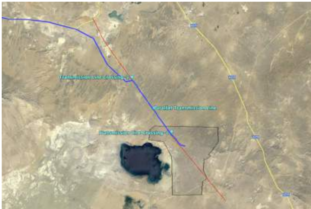
Figure 2-11 OHTL Route Crossing Existing Transmission Line (Ref OHTL Route in Blue and Transmission Line in Red)
