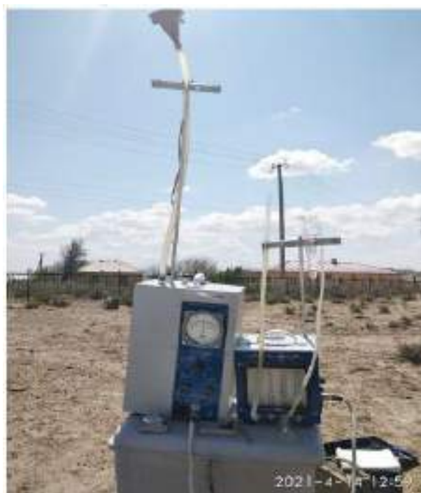
Plate 8-1 Air Quality Monitoring Device Used for Monitoring at the Project Site
