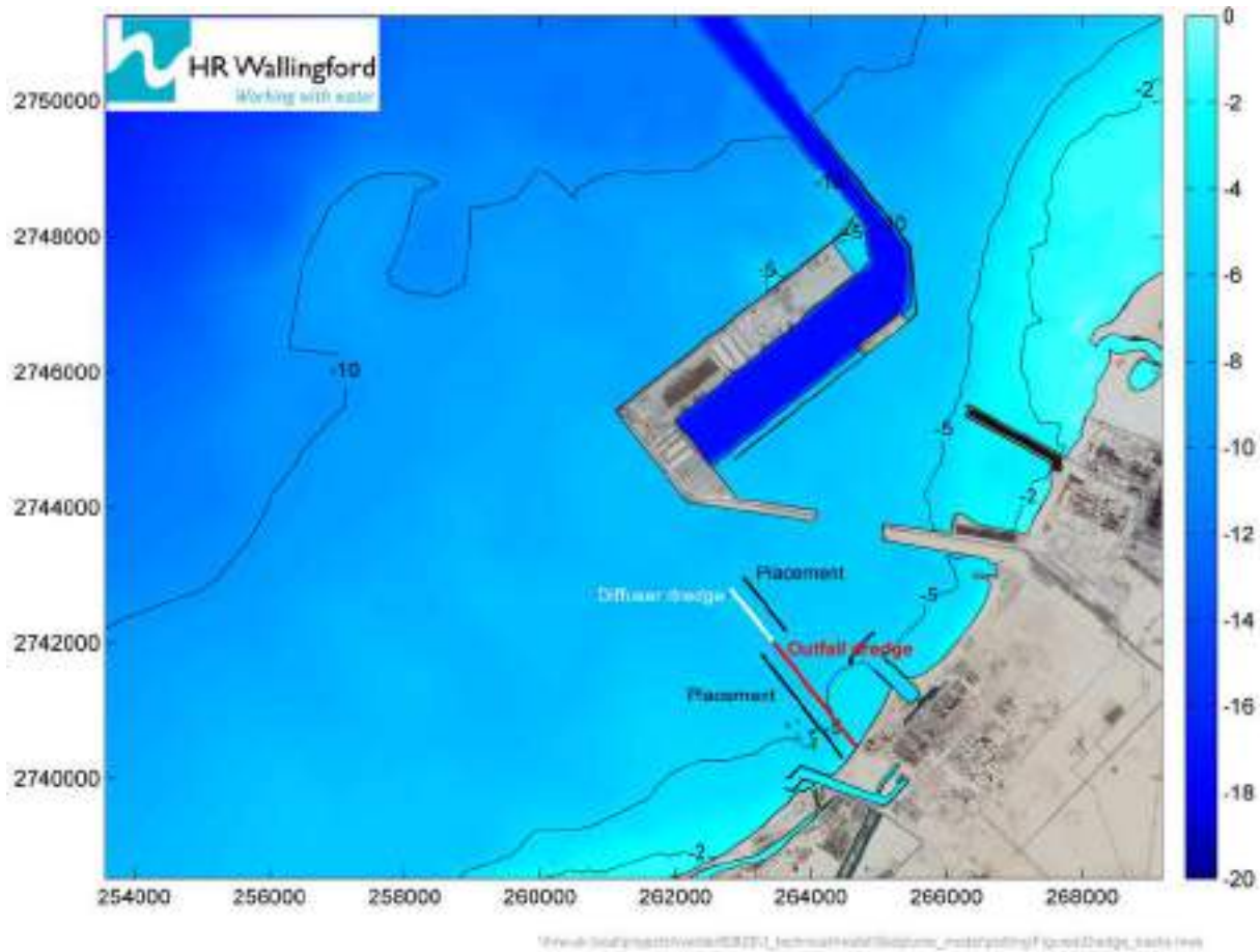
Figure 5-78 Alignment of Dredging and Excavated Material Placement Zones
