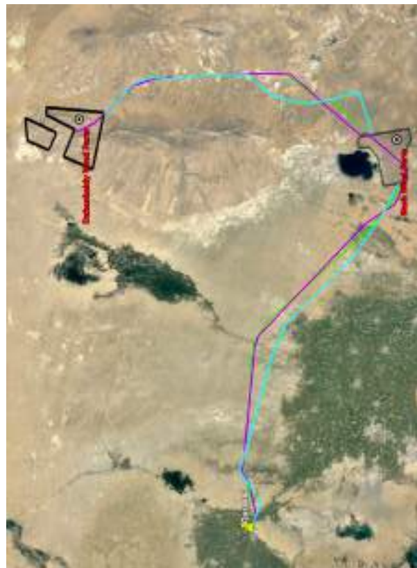
Figure 4-3 The three (3) OHTL Alignment Options – May 2021
