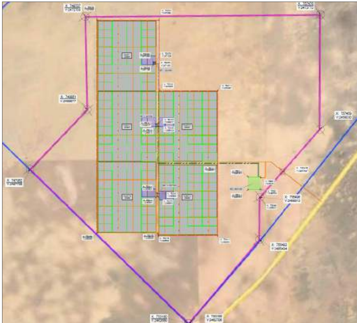
Figure 4 : Solar Power Plant layout
