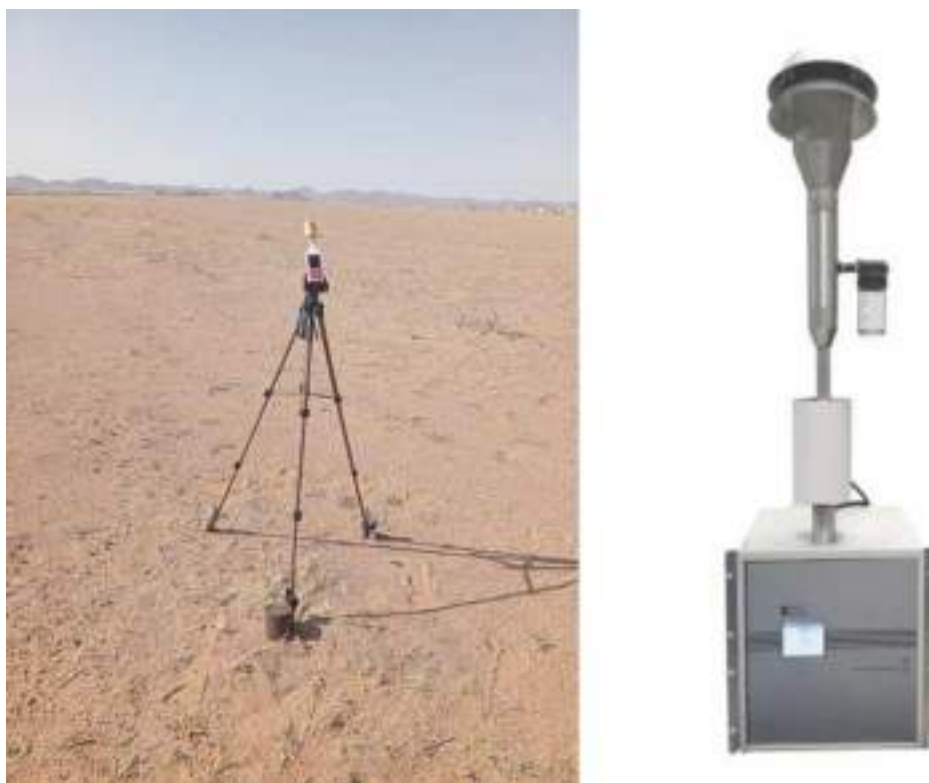
Figure 4.68. Photos showing noise and dust monitoring equipment used in the study.
