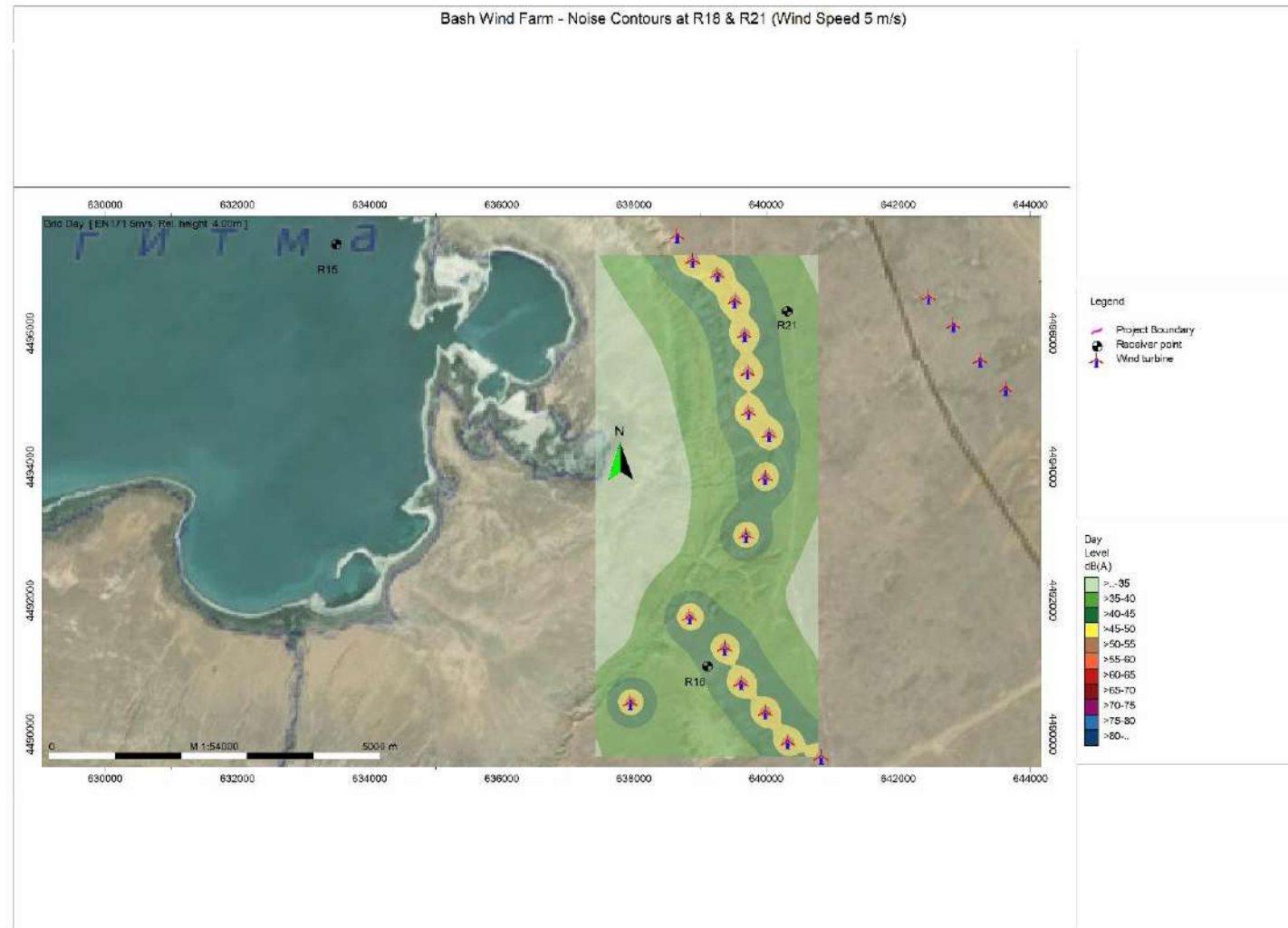
Figure 9-13 Noise Contour at the Project site R18 and R21 (5m/s Wind Speed)
