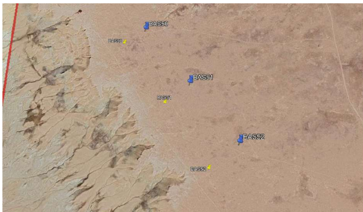
Figure 7-12 Three micrositied turbines maintaining 2km buffer from Lake Ayakagitma
