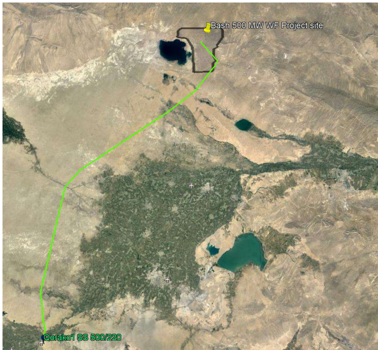
Figure 2-3 Alignment of 162km OHTL from the Bash Wind Farm to Karakul Substation
