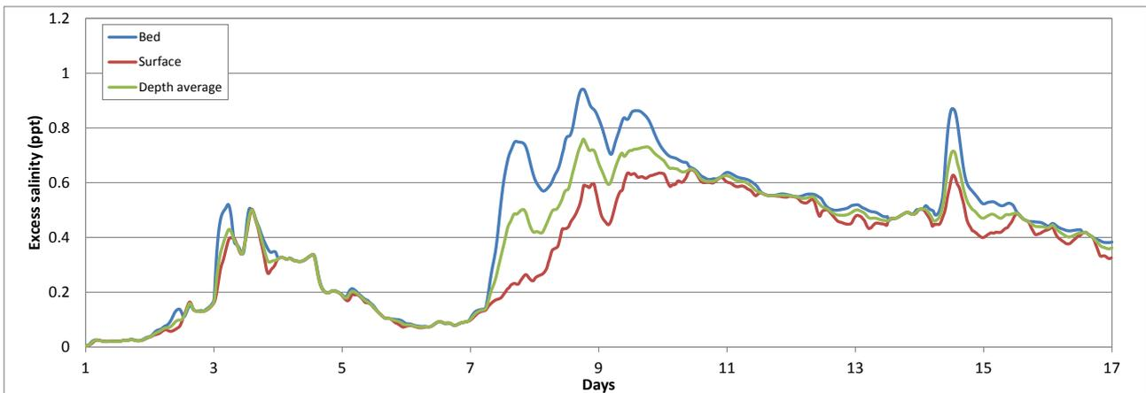
Figure 5.38: Predicted excess salinity at the intakes, stronger winds, open intake layout
