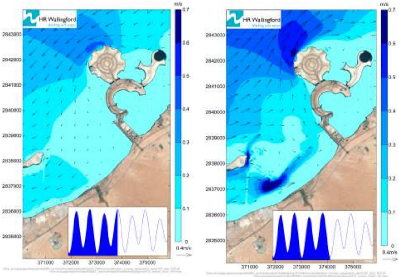
Figure 3.7 Predicted currents, high water, spring tide      Figure 3.8: Predicted currents, low water, spring tide
