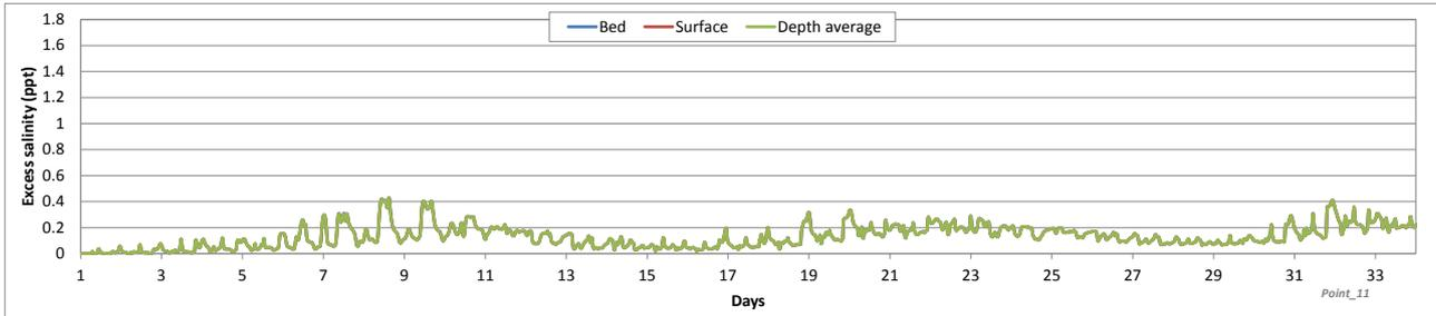
Figure 5.59: Predicted excess salinity at point 11 (Area of Observed Turtles), weak winds, open intake layout
