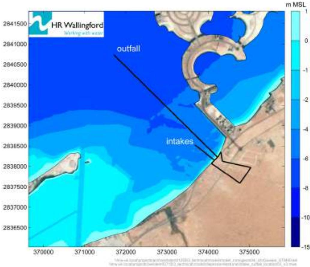
Figure 5.1: Initial intake and outfall locations
