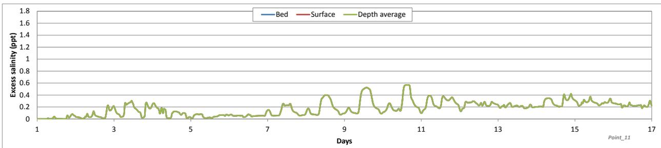
Figure 5.60: Predicted excess salinity at point 11 (Area of Observed Turtles), stronger winds, open intake layout
