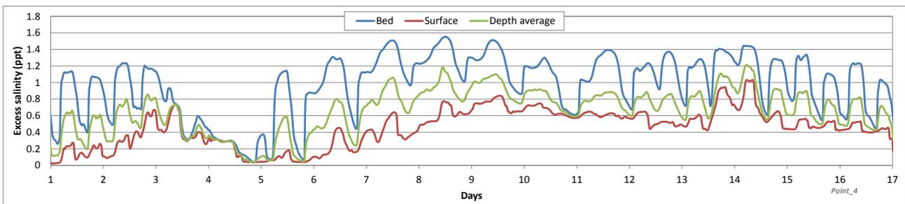
Figure 5.17: Predicted excess salinity at point 4 (tidal channel), stronger winds
