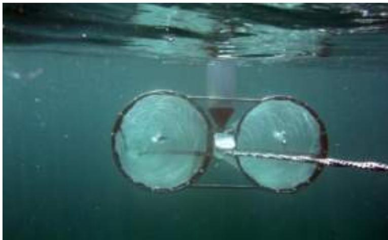
**Lateral view of the 'Bongo' net assembly in operation, showing float attachment and discrete sampling depth (NEA File photo);**
