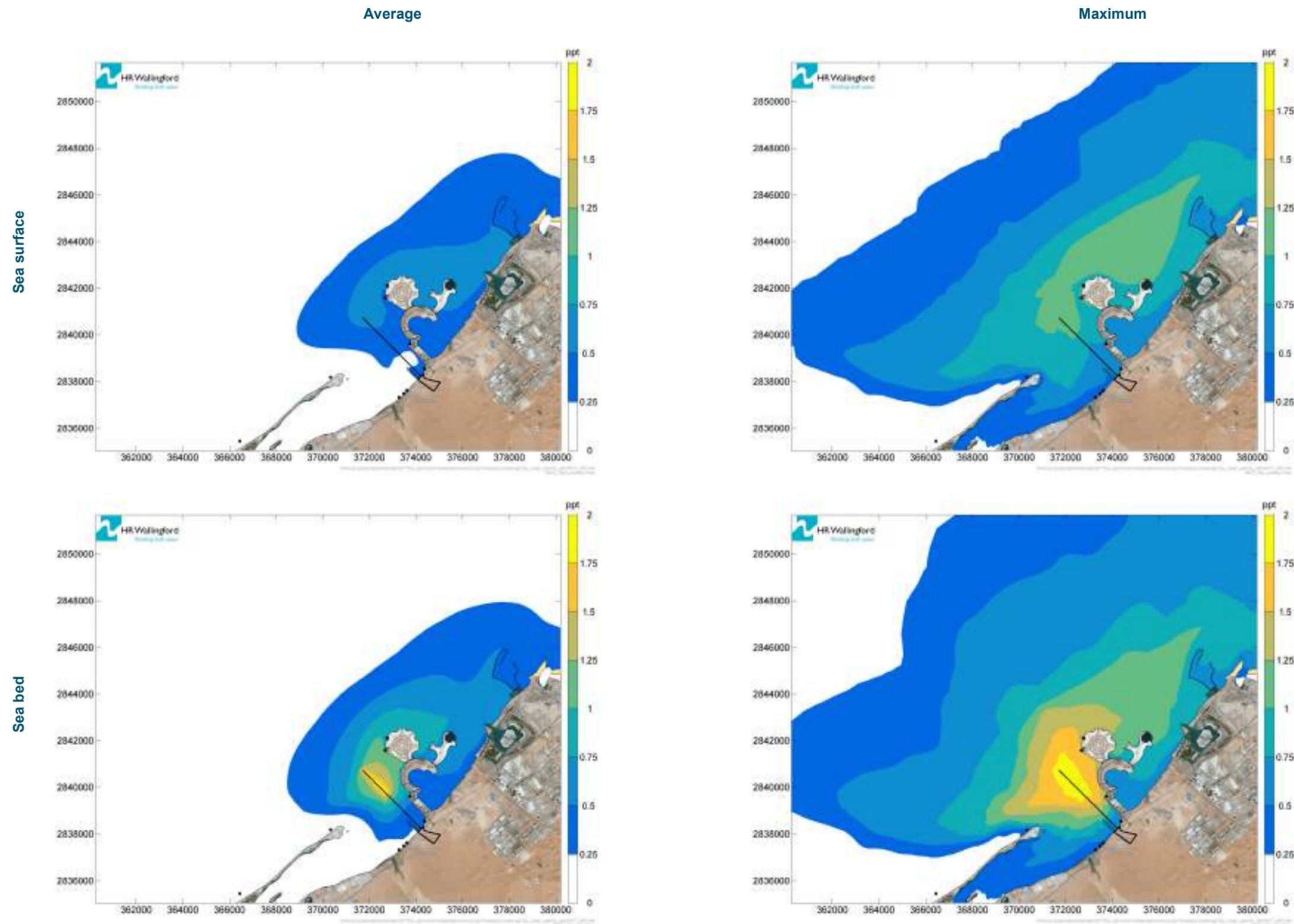
Figure 5.35: Predicted maximum and average excess salinity, weak winds, open intake layout
