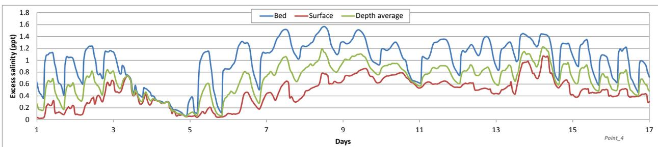
Figure 5.46: Predicted excess salinity at point 4 (tidal channel), stronger winds, open intake layout
