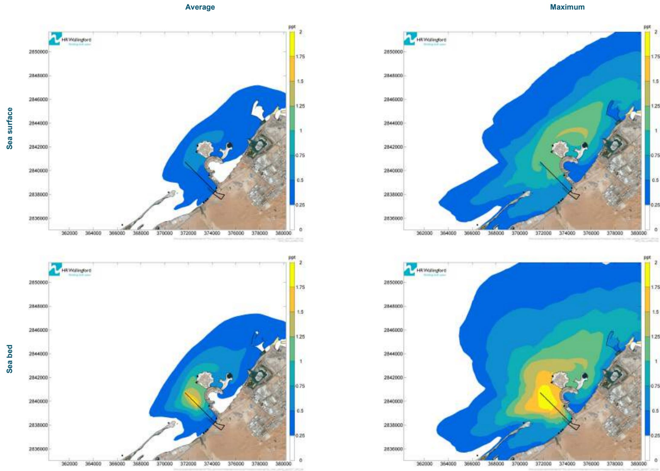
Figure 5.36: Predicted maximum and average excess salinity, stronger winds, open intake layout
