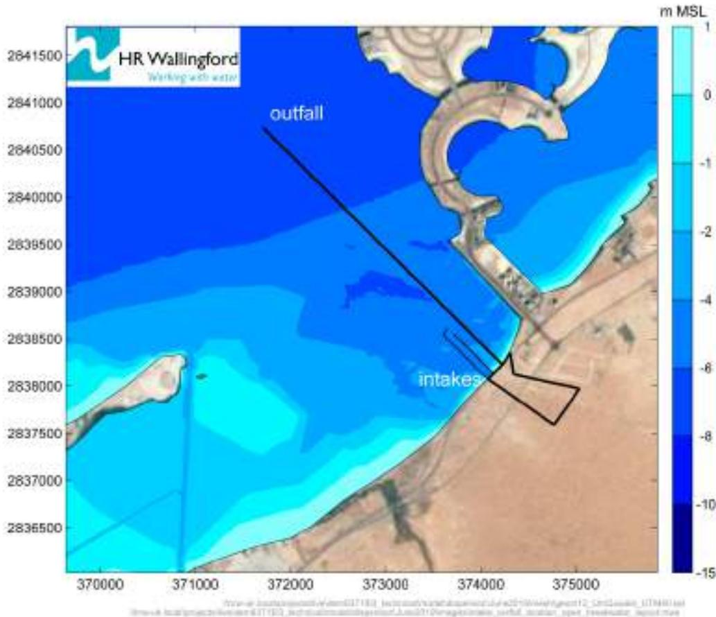
Figure 5.34: Model bathymetry, open intake layout with breakwaters
