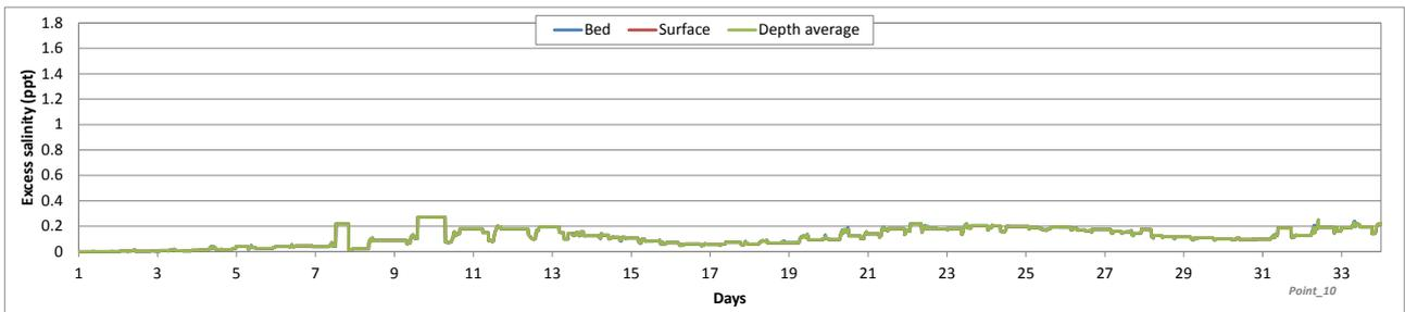
Figure 5.57: Predicted excess salinity at point 10 (Residential Compound 5), weak winds, open intake layout
