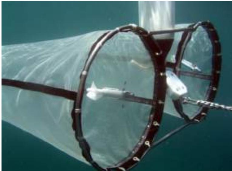
**Close-up view of the 'Bongo' net assembly with flow-meters in place (NEA File photo);**
