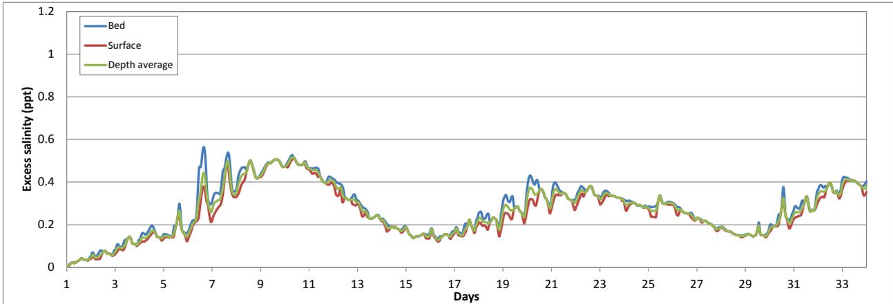
Figure 5.37: Predicted excess salinity at the intakes, weak winds, open intake layout
