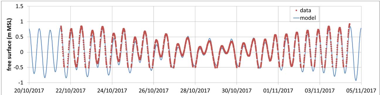
Figure 3.4: Observed and predicted free surface elevation at the ADCP location
