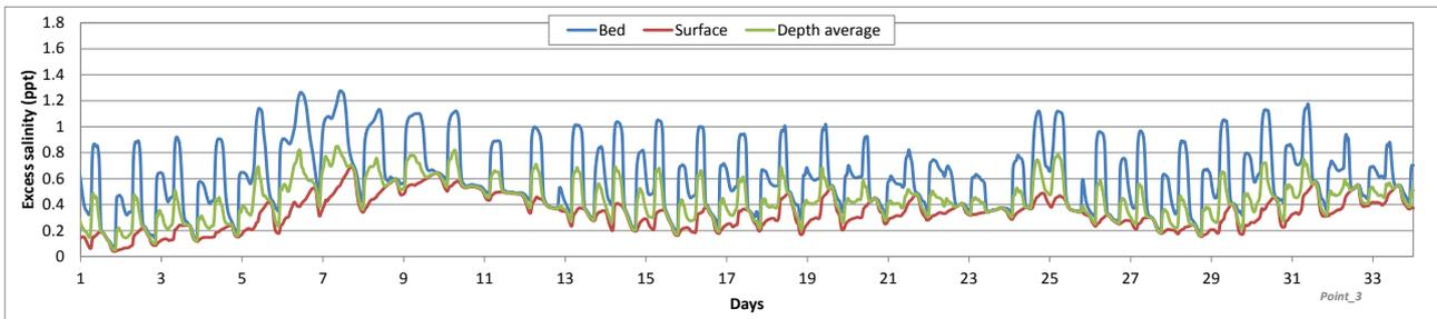
Figure 5.43: Predicted excess salinity at point 3 (Ras Al Khaimah Convention Centre), weak winds, open intake layout
