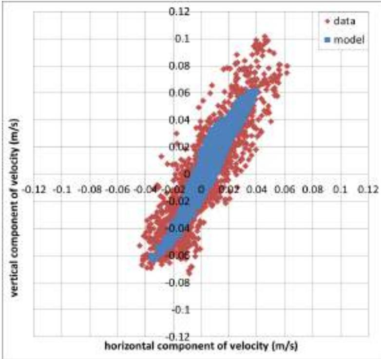
Figure 3.6: Observed and predicted current velocity components at the ADCP location
