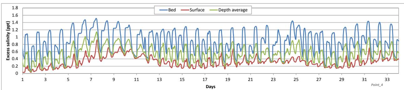
Figure 5.45: Predicted excess salinity at point 4 (tidal channel), weak winds, open intake layout
