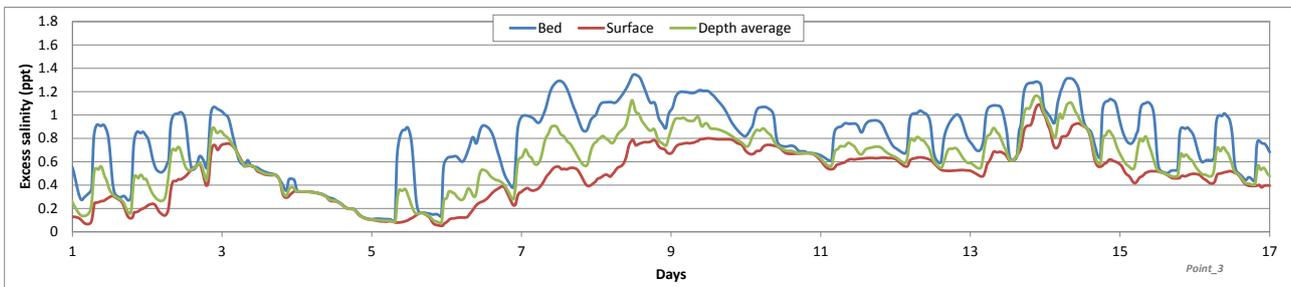
Figure 5.44: Predicted excess salinity at point 3 (Ras Al Khaimah Convention Centre), stronger winds, open intake layout
