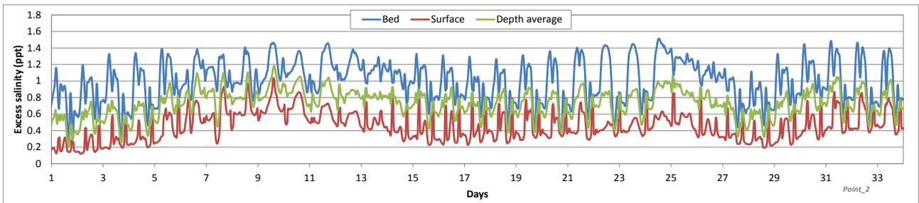
Figure 5.41: Predicted excess salinity at point 2 (Pacific Development), weak winds, open intake layout
