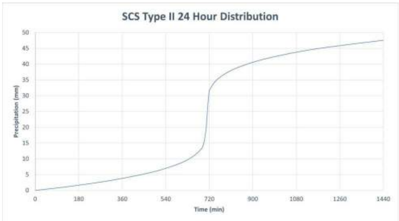
Figure 8-11 SCS Type 2 Rainfall Distribution Curve
