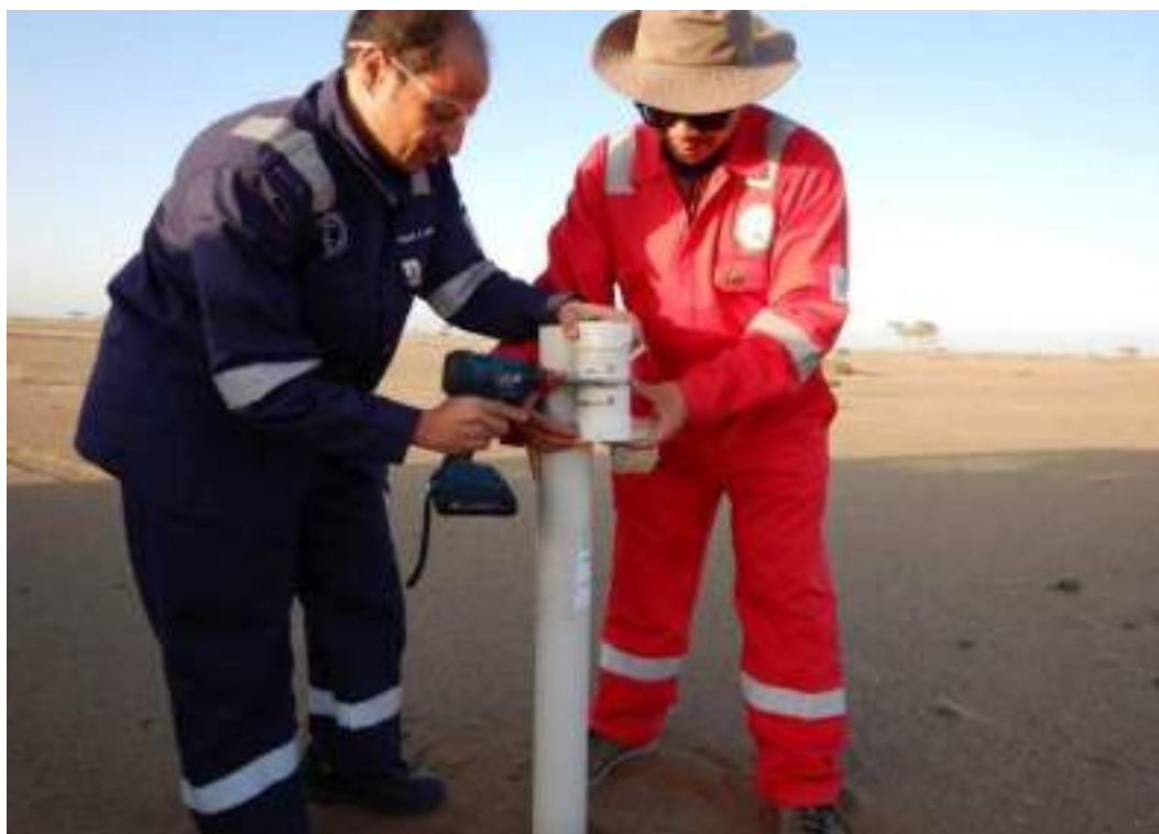
Figure 4.8. Setting up the SQM-LU-DL equipment to measure night sky brightness in Khulais, Makkah, on March 4-12, 2024.
